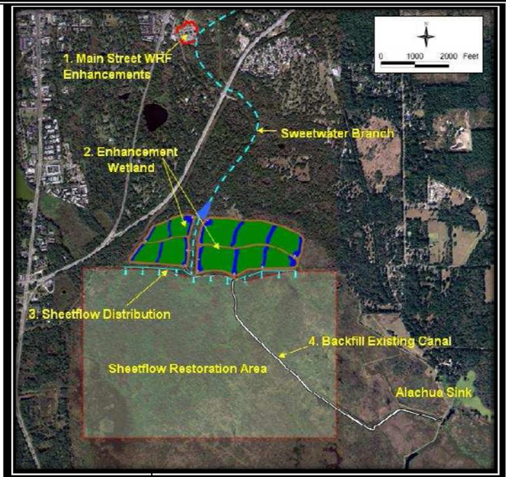
innovative approach to achieving TMDL requirements, 4) construction of a 1.25 mile long sheetflow distribution channel, and 5) back fill approximately one mile of existing canal to eliminate short circuiting.
