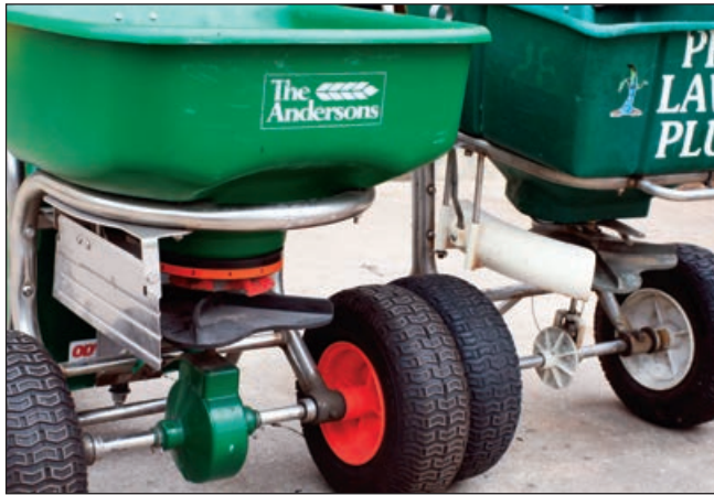
Figure 21. Spreaders with deflector shields.
