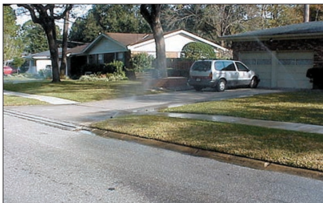
Figure 9. Overirrigation, runoff. Small turf area should be irrigated with spray heads, not sprinklers.
