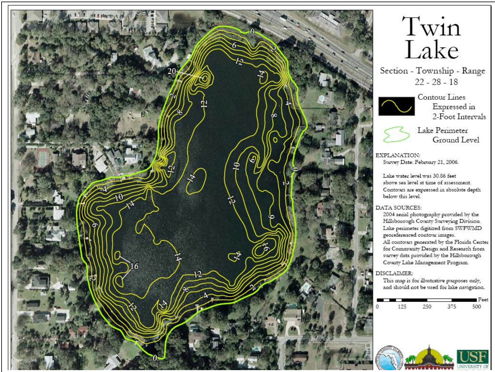
Figure 1. Contour map for Twin Lake created in 2006. The mapping technique used in 2008 employs a standard DGPS for horizontal position and a fathometer for depth.
