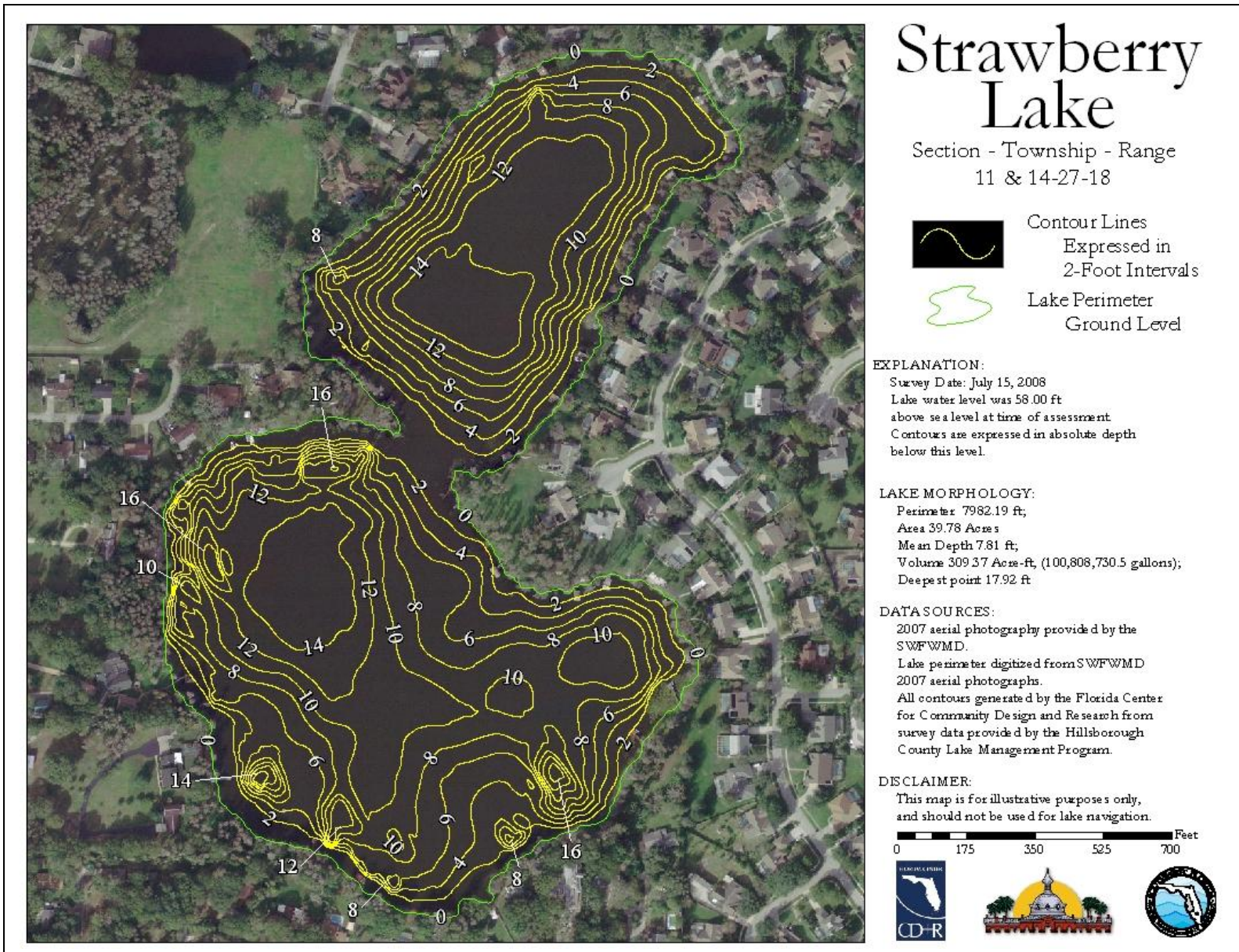
Figure 1. Contour map for Strawberry Lake. The mapping technique used in 2008 employs a standard DGPS for horizontal position and a fathometer for depth.
