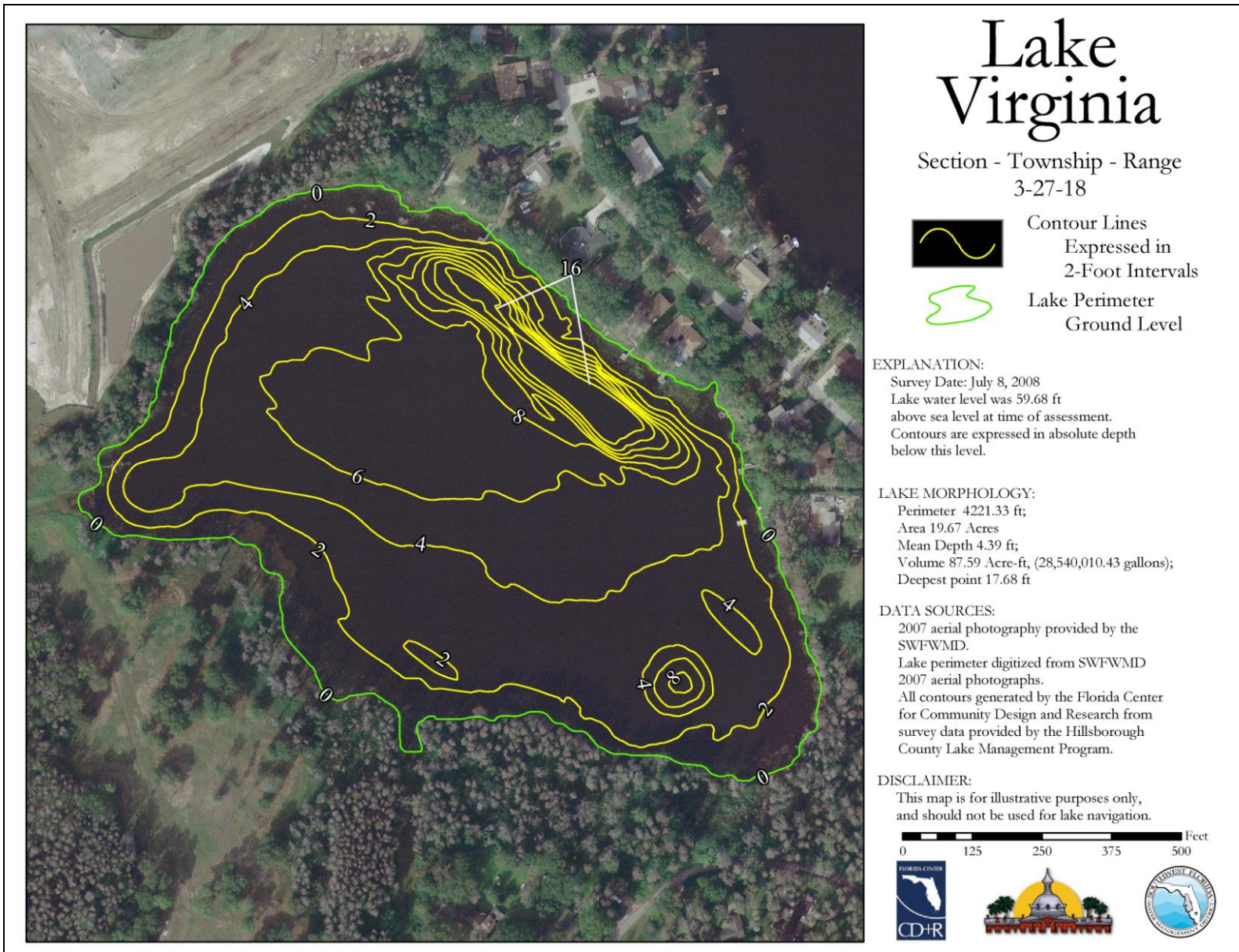
Figure 1. Contour map for Lake Virginia. The mapping technique used in 2008 employs a standard DGPS for horizontal position and a fathometer for depth.
