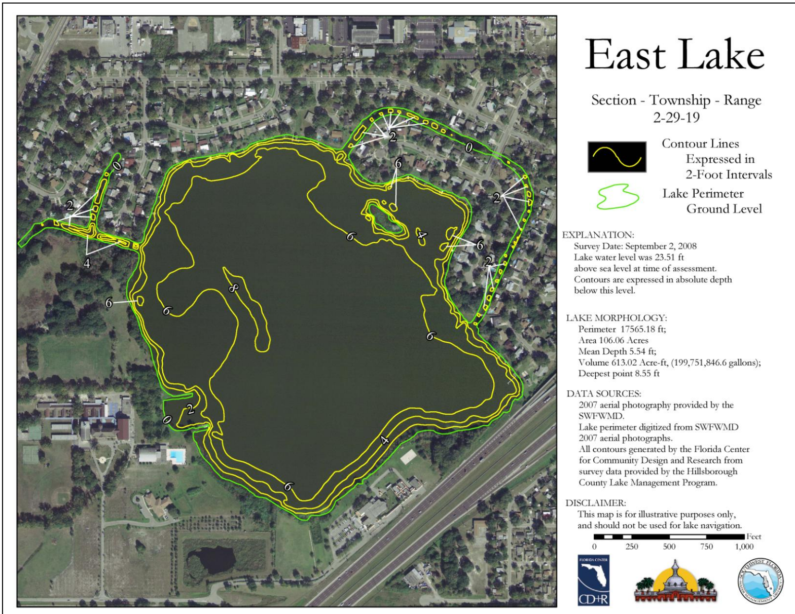
Figure 1. Contour map for East Lake. The mapping technique used in 2008 employs a standard DGPS for horizontal position and a fathometer for depth.
