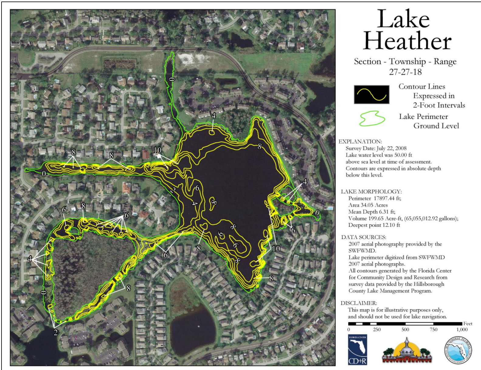
Figure 1. Contour map for Lake Heather. The mapping technique used in 2008 employs a standard DGPS for horizontal position and a fathometer for depth.
