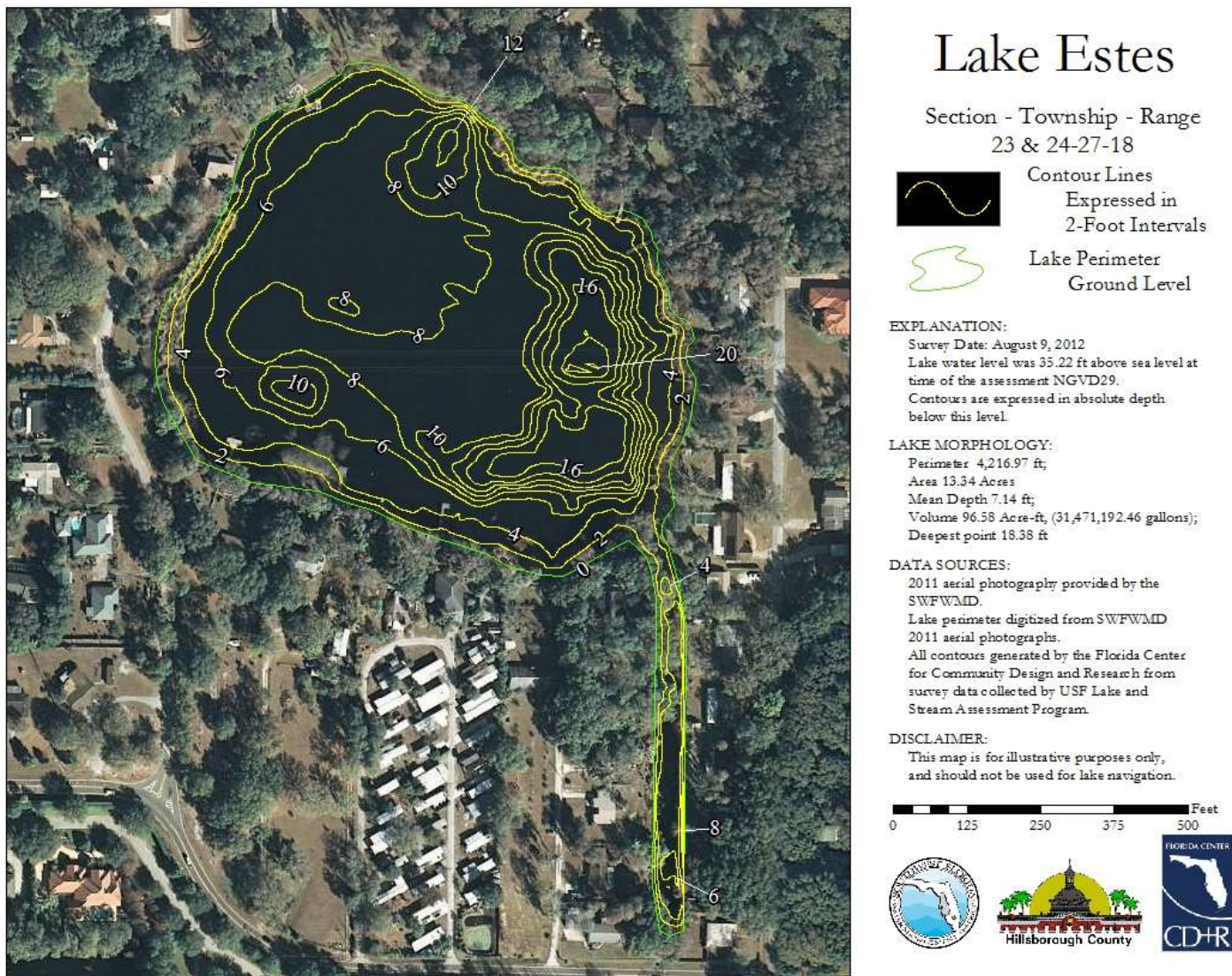
Figure 2. Bathymetric contour map for Lake Estes created from data collected during the 2012 lake assessment.
