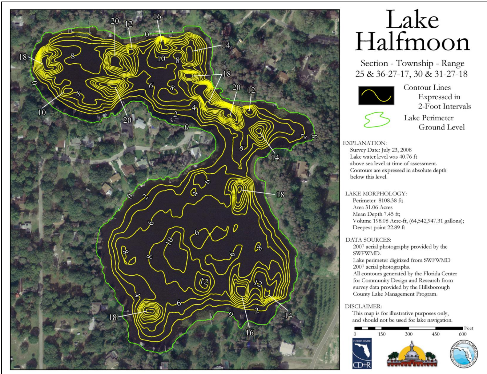
Figure 1. Contour map for Half Moon Lake. The mapping technique used in 2008 employs a standard DGPS for horizontal position and a fathometer for depth.
