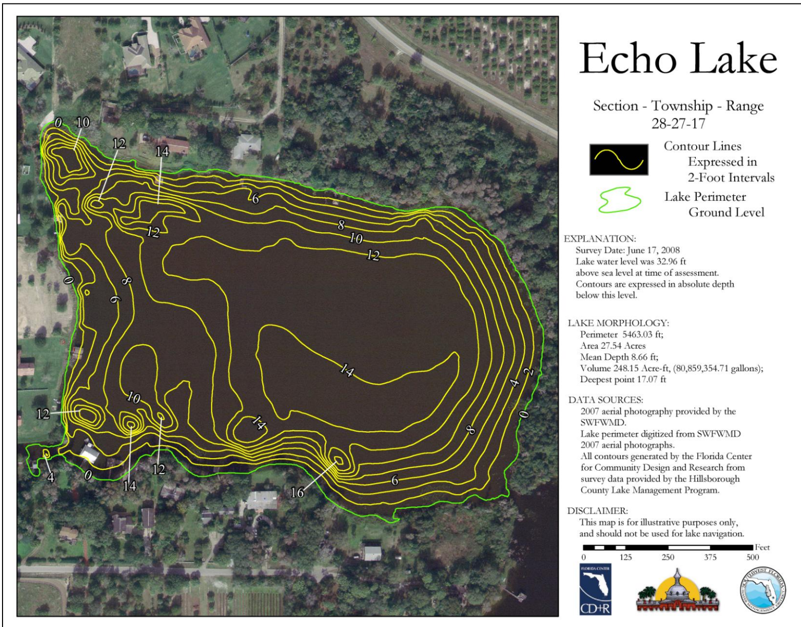
Figure 1. Contour map for Echo Lake. The mapping technique used in 2008 employs a standard DGPS for horizontal position and a fathometer for depth.
