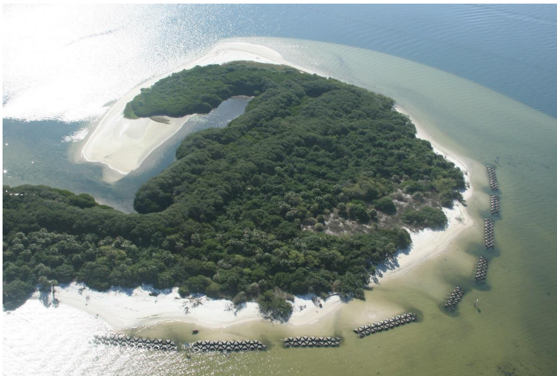
Figure 32. Concrete pyramid oyster reef habitat installed on north and west sides of Sunken Island.
