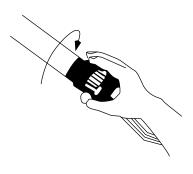
C. Apply new joint sealer or tape, using package instructions. Use adjustable wrench to install new showerhead.
