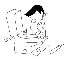
C. Apply grout where the toilet meets floor to give it a finished look. Smooth the grout bead with a wet finger. Re-connect the supply line, fill the tank and flush to test.
