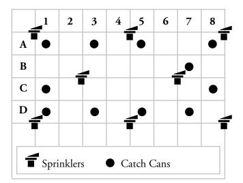
4. Turn on the system or zone for 7 to 10 minutes for a spray head zone or 20 to 40 minutes for a rotor zone. Visually check the cansduring the test to see if a measurable amount of water has collected; if not, run the system longer, recording the time.
