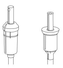
▲ Sprinklers are categorized as spray heads or rotors. Spray heads apply water at relatively high rates (1.5 in./hr.) to the immediate area, while rotors use 2 to 3 times less water, and irrigate larger areas. Therefore, spray zones are operated for shorter durations than rotor zones.
