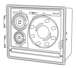
▲ The **controller** is an electronic or mechanical timer connected to a series of valves to turn the system on and off at specified intervals. Each area watered by a control valve is called a zone. Electronic controllers are often preferred because they allow different operating schedules for each zone. Not knowing how to operate or adjust the controller leads to the greatest waste of water.
