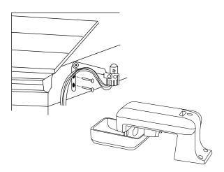
▲ The rain shutoff device keeps the irrigation system from operating when rainfall accumulation reaches a pre-set level. They are designed to interrupt the flow of electricity to the pumps, so that the timer in the controller does not need to be reset. Florida law requires that all automatic inground irrigation systems (installed after May 1, 1991) be equipped with an automatic rain shutoff device.
