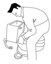
A. Close the supply valve. Flush the toilet, unscrew supply line and hold-down nuts. Remove lid to lessen weight and remove toilet.
