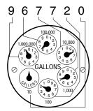
2. Round reading meters read like a clock with some of the dials turning counterclockwise. Check the numbers to determine the direction of the turning dial. Start with the highest numbered dial (100,000) then the next (10,000) then the next (1,000) until you have read all dials. Add these numbers together to determine the current reading.
