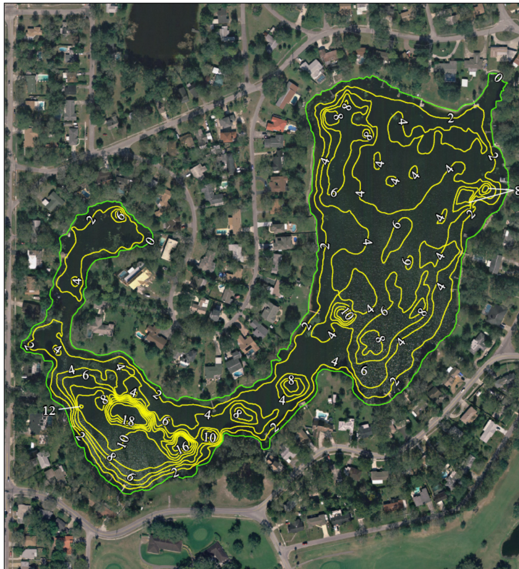
Figure 1. . Contour map for Lake Eckles. The mapping technique used in 2006 employs a standard DGPS for horizontal position and a fathometer for depth.
