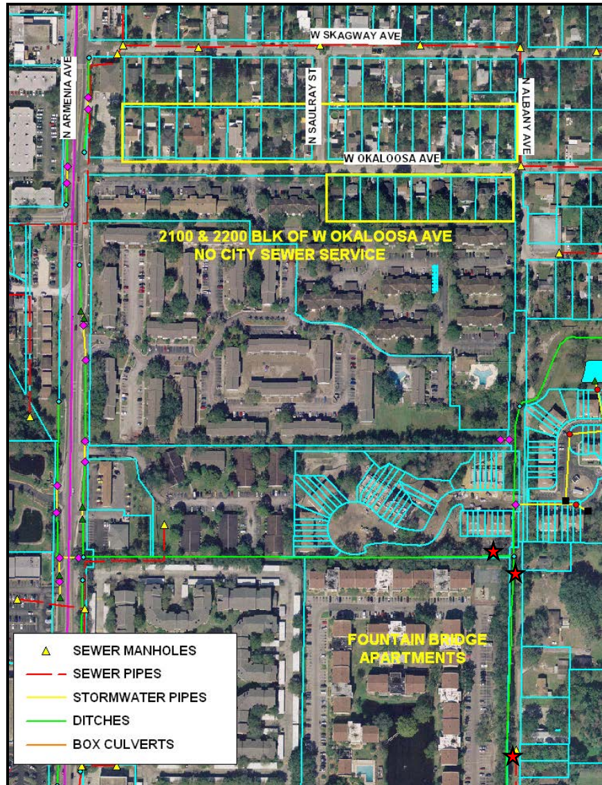
Map 17. Parcels, outlined in yellow, located upstream of stations DHR7, DHR8, DHR9, and DHR10, identified by the COT as not having an existing sanitary sewer account. This map was provided by the COT (November 28, 2007). The red stars indicate the approximate locations of stations DHR7, DHR8, and DHR9. Blue lines denote parcel boundaries.
