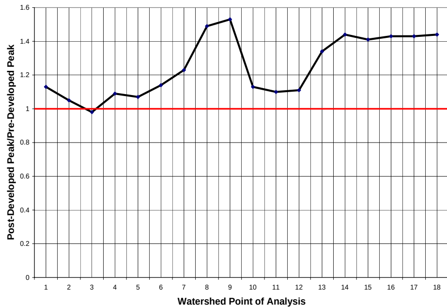
Figure 10-3: Comparison of 2-Year Pre- and Post-Developed Peak Rates with Peak Rate Controls, Devils Brook Watershed
