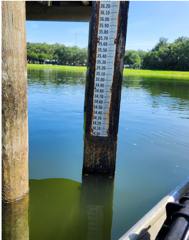
Figure 4 Gauge note height showing below normal levels at Gornto Lake
