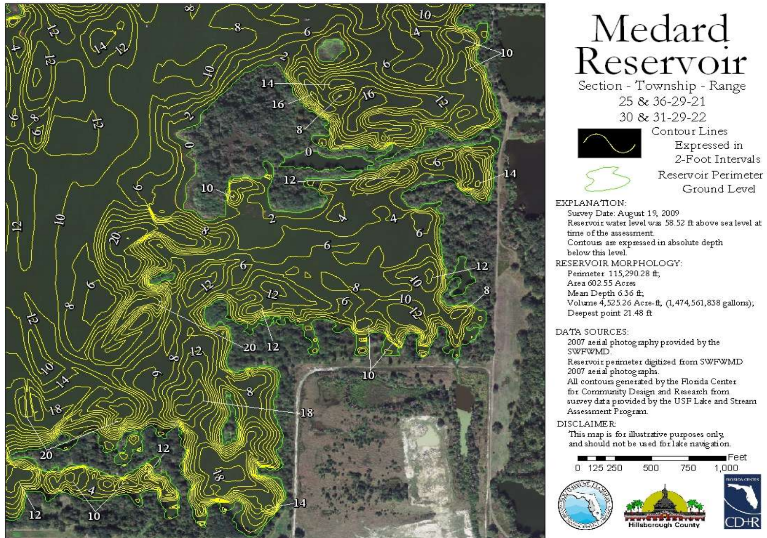
Figure 6. Contour map for Medard Reservoir (southeast). The mapping technique used in 2009 employs a standard DGPS for horizontal position and a fathometer for depth.
