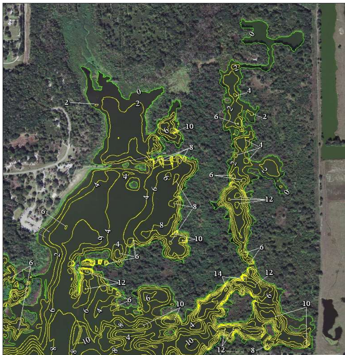
Figure 3. Contour map for Medard Reservoir (northeast). The mapping technique used in 2009 employs a standard DGPS for horizontal position and a fathometer for depth.
