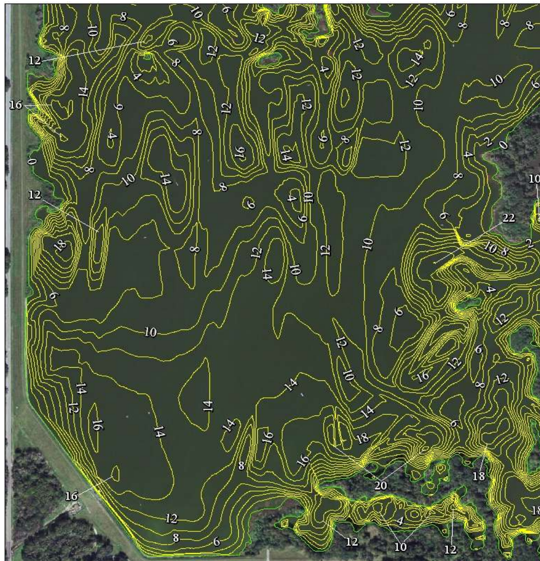
Figure 5. Contour map for Medard Reservoir (southwest). The mapping technique used in 2009 employs a standard DGPS for horizontal position and a fathometer for depth.
