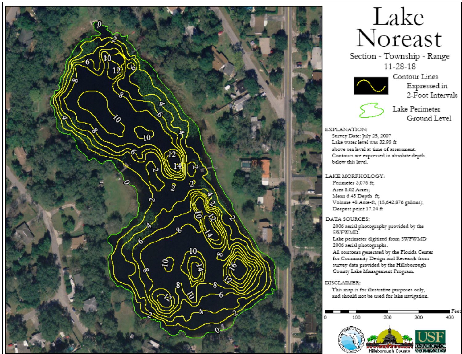
Figure 1. Contour map for Lake Noreast. The mapping technique used in 2007 employs a standard DGPS for horizontal position and a fathometer for depth.
