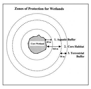
In this diagram of zones of protection for wetlands, both core habitat and aquatic buffer requirements are met within a 164-meter zone. An additional 50-meter buffer is recommended to protect core habitat.
