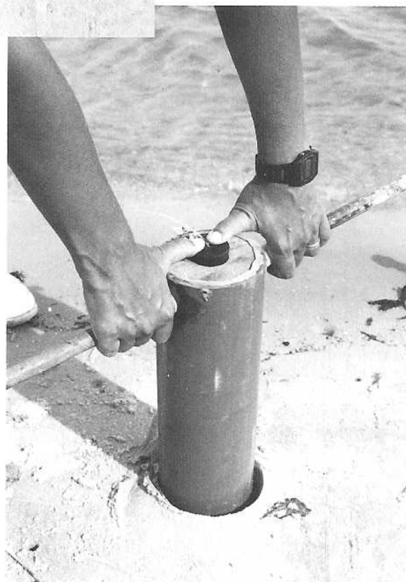
Figure 2. Demonstration of core tube on sand beach. Planting on beach for demonstration only. (Top) 4-inch diameter PVC core tube with 1-inch PVC tube installed and sealed. Removable metal handle inserted in tube for coring. Rubber stopper loose on top for insertion into sediment. Note beveled lower edge of 4-inch tube to aid in cutting rhizomes. (Right) Core tube after twisting into sediment to depth of ca. 20 cm. Rubber stopper is in place in plywood plug that was screwed in place and bedded in sealant. Placement of the stopper creates a vacuum that allows the plug of seagrass to be withdrawn from the substrate. Removal of the stopper allows the plug to slide out of the tube into the substrate for planting.
