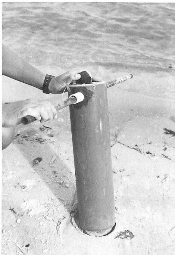
Figure 2. Demonstration of core tube on sand beach. Planting on beach for demonstration only. (Top) 4-inch diameter PVC core tube with 1-inch PVC tube installed and sealed. Removable metal handle inserted in tube for coring. Rubber stopper loose on top for insertion into sediment. Note beveled lower edge of 4-inch tube to aid in cutting rhizomes. (Right) Core tube after twisting into sediment to depth of ca. 20 cm. Rubber stopper is in place in plywood plug that was screwed in place and bedded in sealant. Placement of the stopper creates a vacuum that allows the plug of seagrass to be withdrawn from the substrate. Removal of the stopper allows the plug to slide out of the tube into the substrate for planting.
