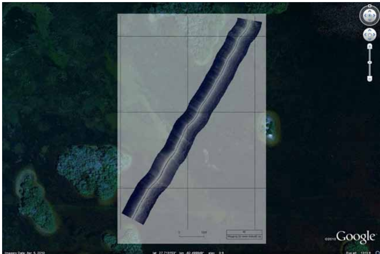
Figure 23. The output of a sidescan assessment of CB03 transect. The chart analyzed with the Dr. Depth software and displayed as a KML feature in Google Earth.
