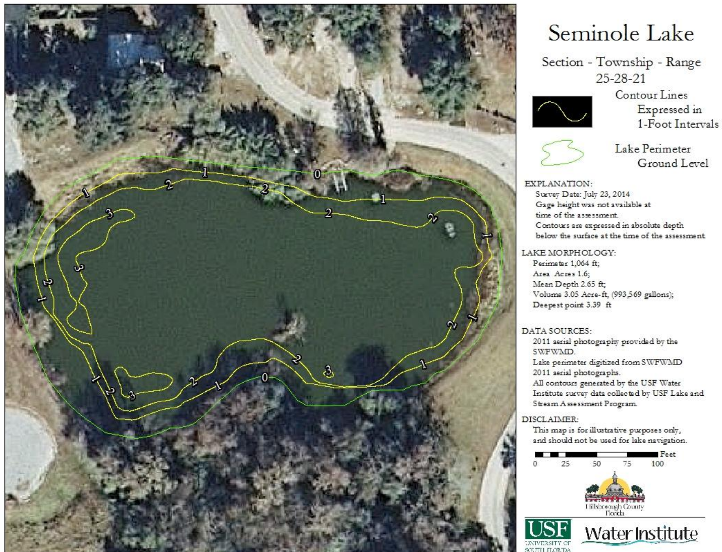
Figure 2. 2014 2-Foot Bathymetric Contour Map for Seminole Lake
