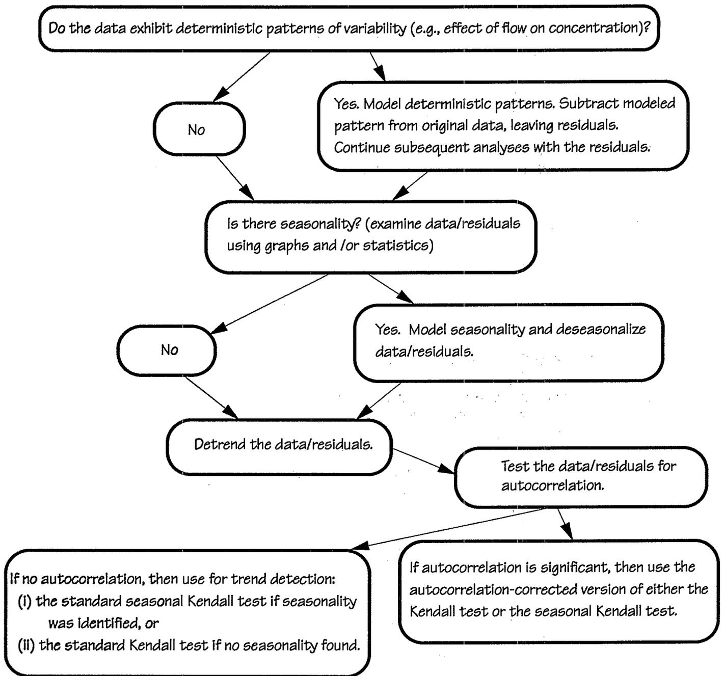
Figure 3.8. Data analyses used to identify the appropriate test for trend detection.
