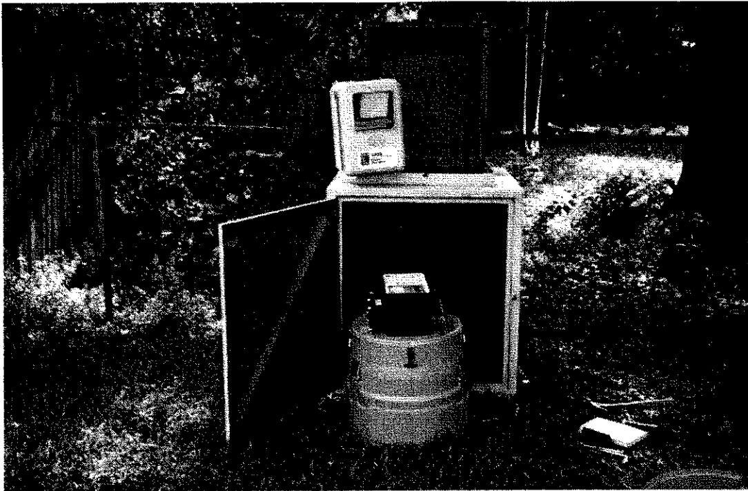
Photo 3 ISCO Automatic Sampling Equipment used during study
