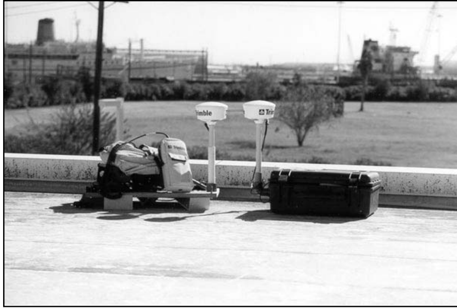
Figure 3. Trimble Pathfinder PRO XR instruments located on the roof of the City of Tampa Bay Study Group laboratory during tests of vertical measurement errors.
