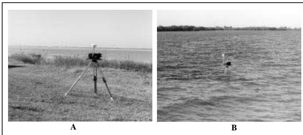
Figure 7. Field set-ups of base (A) and rover (B) stations during GPS seagrass elevation measurements in Tampa Bay.
