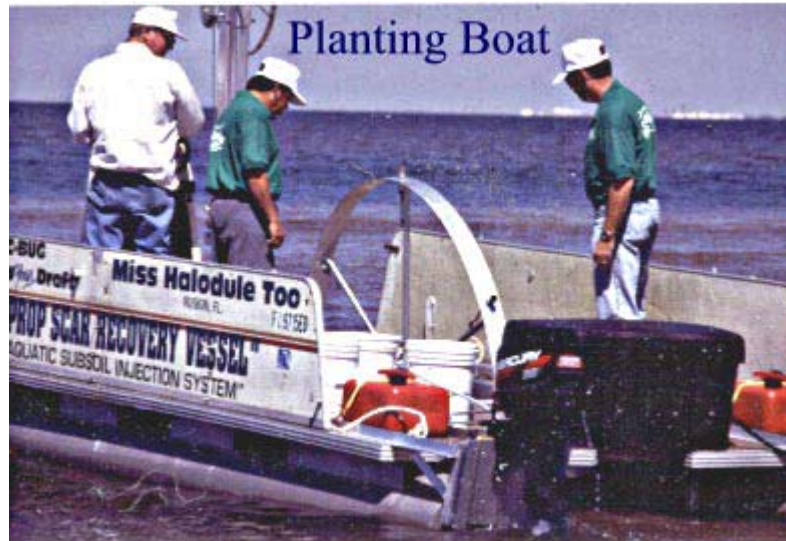
Figure 3. Anderson's planting boat. Note the planting wheel in the center.
