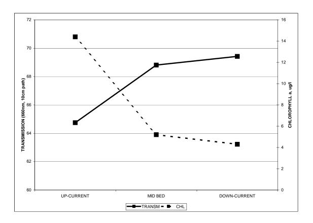
Figure 4. Surface chlorophyll a concentrations and percent light transmission (C-Star<sup>®</sup> transmissometer at 660nm, 10cm path length) measured at the CP1 green mussel bed at Catfish Point in March 2003. Samples were collected up-current from the bed, in the center of the bed, and down-current from the bed during an incoming tide.
