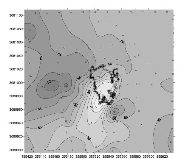
Figure 5. Contour plot showing percent light transmission (C-Star® transmissometer at 660nm, 10cm path length) at the CP1 green mussel bed at Catfish Point. Lighter gray shade indicates higher light transmission. The perimeter of the main portion of the bed (+), mapped in March 2003, and light transmission measurement sites (o), from June 2003, are also shown. Both were determined with DGPS. Axes units are UTM meters.
