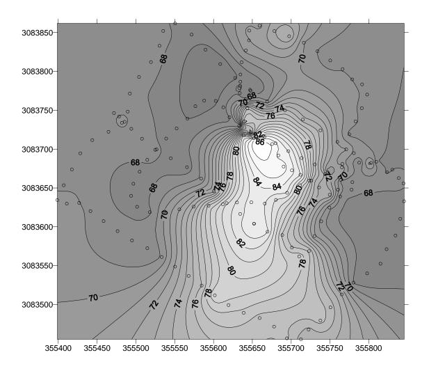
Figure 6. Contour plot showing percent light transmission (C-Star® transmissometer at 660nm, 10cm path length) at the Long Shoal green mussel bed in July 2003. The bed has not yet been mapped, however, the main portion of the bed is located in the center of the graph. Lighter gray shade indicates higher light transmission. Light transmission measurement sites (o) were determined with DGPS. Axes units are UTM meters.
