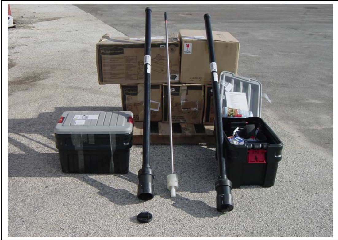
Figure 3. Photo of the ChevronTexaco spill sampling kit located at the Chevron Port Tampa fuel terminal.
