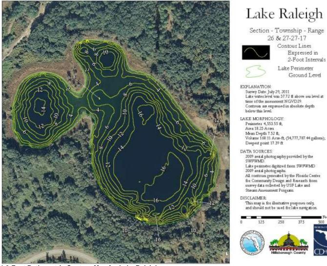
Figure 2. 2011 2-Foot Bathymetric Contour Map for Lake Raleigh
