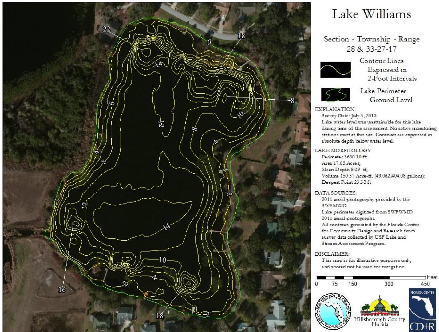
Figure 2. 2013 2-Foot Bathymetric Contour Map for Lake Williams
