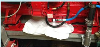
Oil absorbant booms, sheets (bottom), and pads can be kept on your boat to catch leaks under the engine or to contain and remove oil at the surface of the water (back). Bilge socks (top) trap any oily overflow on board, making safe disposal easy. (MASGC/Tara Skelton)
